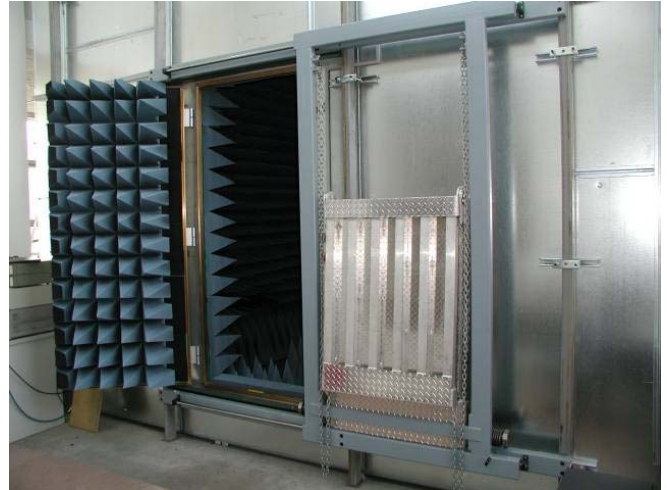
Figure 6. 5m Chamber DUT Access Catwalk
