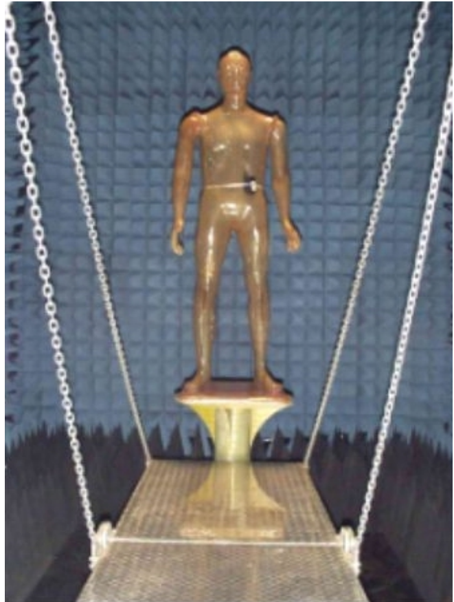
Figure 9. DUT Fixtured on Full Size Human Phantom
